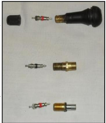
body cleaned up, the threaded end that the dust cap fits on is conveniently 5/16" x 32tpi, which can be used for chucking. A female threaded inserts probably best so everything's concentric. The other end can be turned down and threaded 7/32" x 40tpi as in the bottom of the photo or a brass sleeve could be silver soldered on and threaded to 5/16" x 32tpi as unit in centre of photo. The overall length is not critical but the ones I made were 13/16" long.
