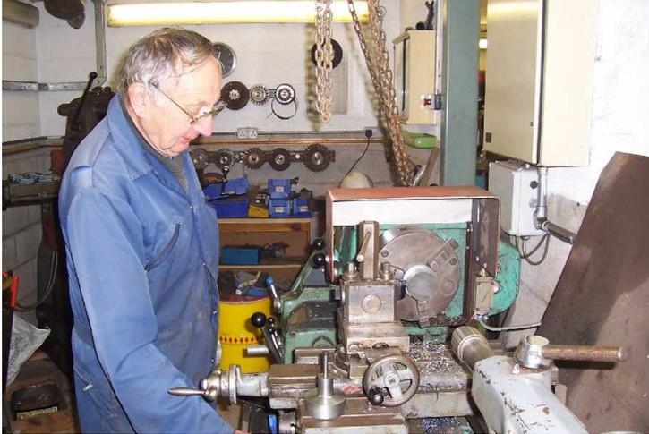
Dave M. machining new buffers for the George Weedon Diesel
