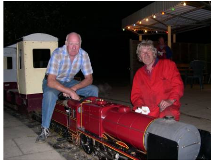
Chris Perkin's new engine Initially a school project, took him 4 years to build, runs well on 7 1/4" ground level.
