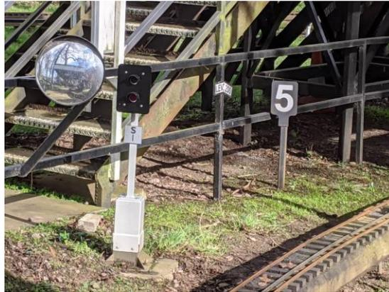
*Examples of line side signal and signage for speed limit and gradient*
